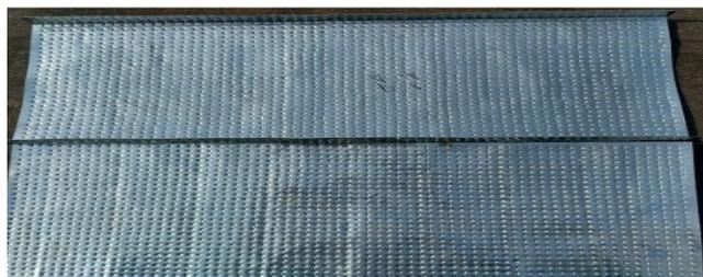
Photograph of three- and one-side roughened absorber plate
