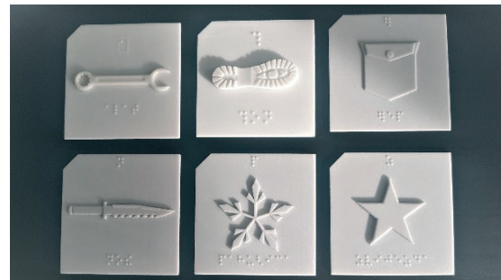
Figure 4: Tiles printed with Spectrum Z 510 3D printer
