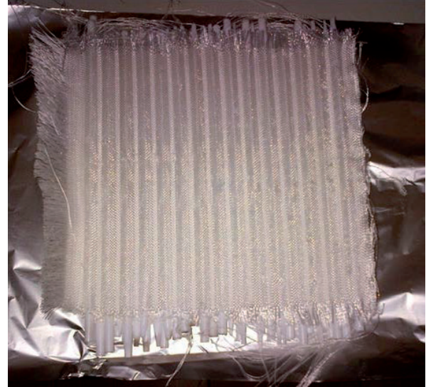
3B. Fabric reinforced with PTFE sticks
