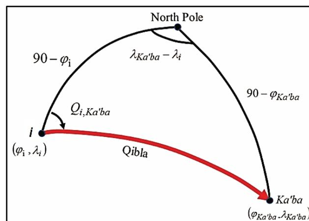
Figure 2 Qibla angle on a spherical triangle
