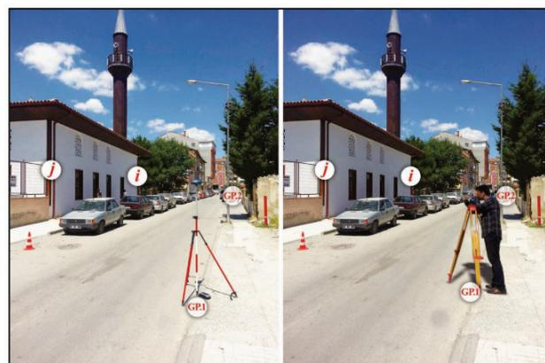
Figure 5 GNSS (left) and conventional (right) measurements
