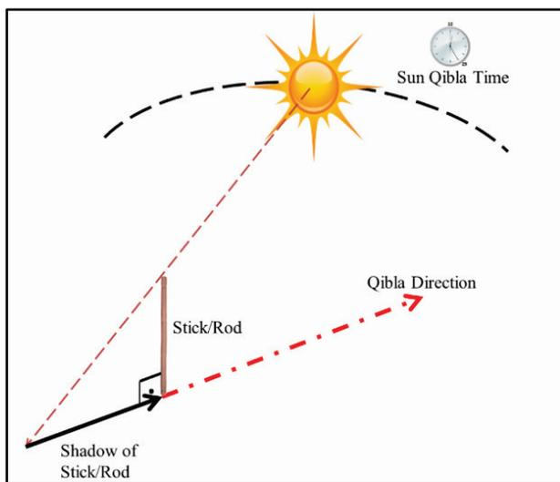
Figure 4 Qibla determination with the sun qibla time method
