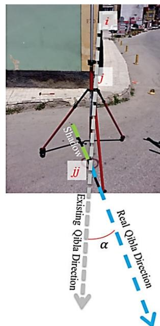
Figure 8 Determination of qibla direction by using sun qibla time
