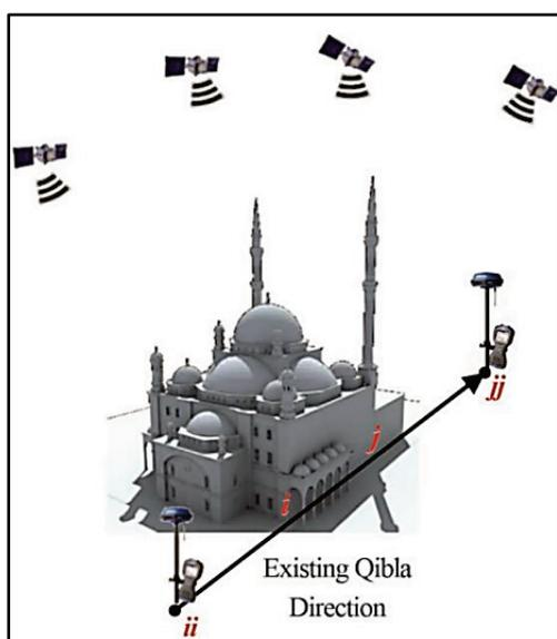
Figure 7 Schematic depiction of field measurement with network-RTK GNSS measurements
