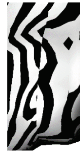
Figure 13 Zebra analysis of NURBS surface clearly shows discontinuity of reflection stripes at the border between adjacent shaft and distal surface segment
