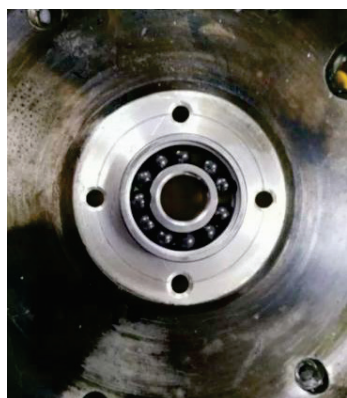
Figure 25 Inner wall of diffuser and bearing seat
