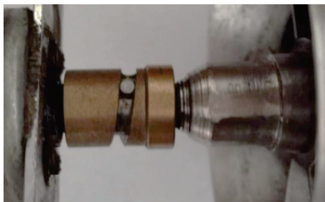
Figure 18 Clutch between engine rotor and starting motor
