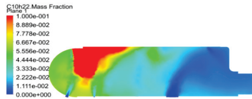
Figure 10 A section of diesel steam mass fraction
