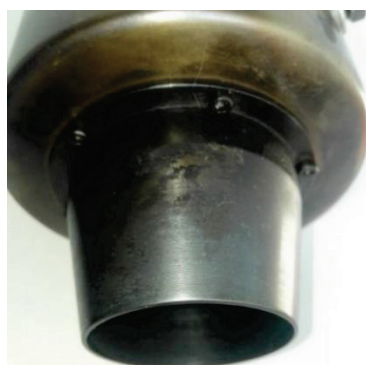
Figure 24 Tail nozzle after combustion
