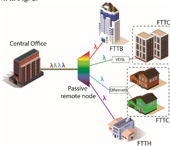
Fig. 2. Structure of WDM-PON
