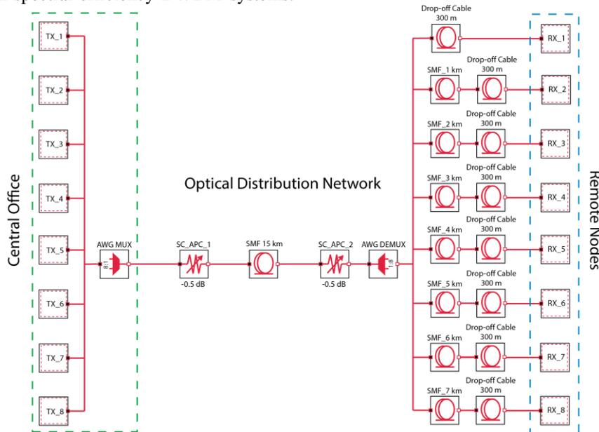
Fig. 5. Structure of proposed 10 Gbps DWDM-PON
