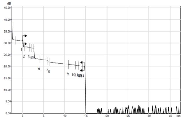
Fig. 8. The reflection curve of the real ODN
