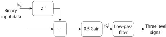
Fig. 4. Duobinary precoder
