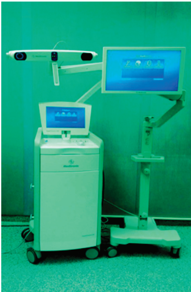
Figure 2. Device for DBS planning, StealthStation S7
