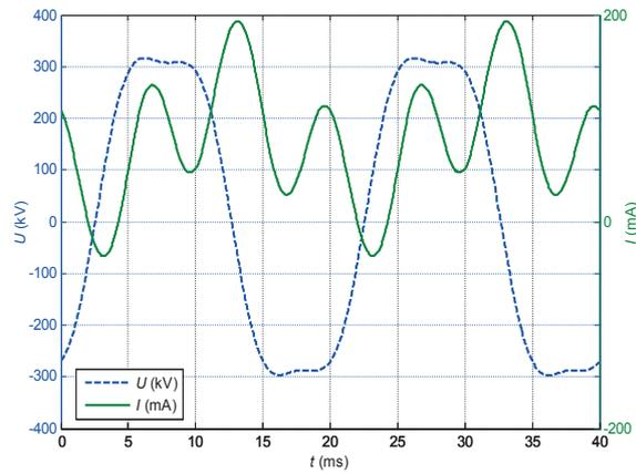
Figure 12.  $U$ - $I$  waveforms for  $I_{DC}=80$  mA
