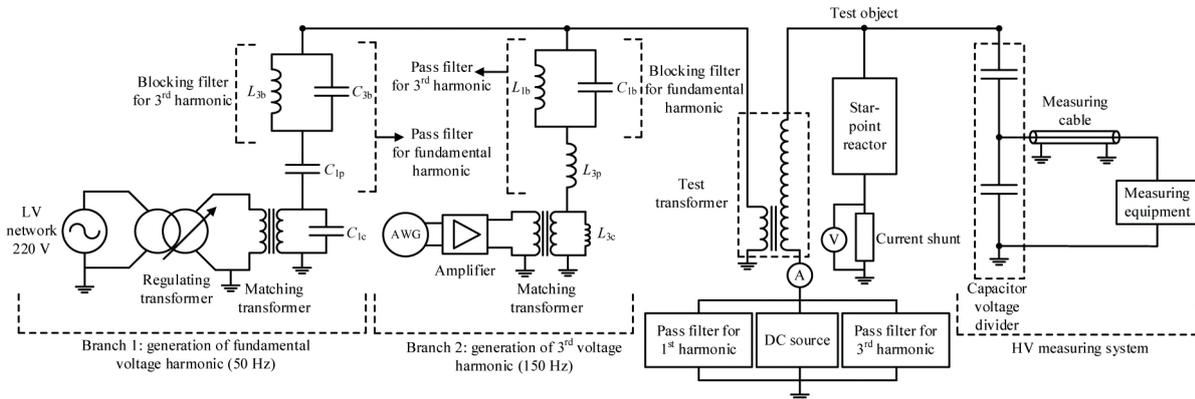
Figure 5. Test circuit for DC current capability test
