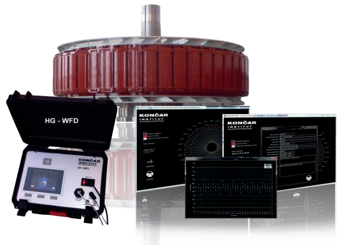
Figure 12. HG-WFD System (Hydro Generator Winding Fault Detection)
