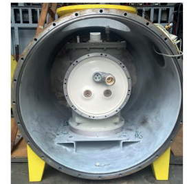
Fig. 5 Internal arc development testing in Končar – High Power Laboratory
