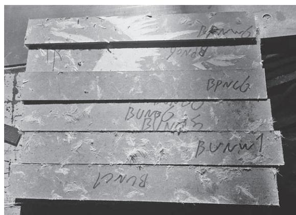
**Figure 2** Surface of MOR specimens with feather content
