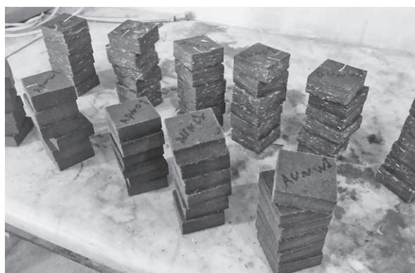
**Figure 1** Water absorption and thickness swelling specimens after being immersed in distilled water for 24 hours
