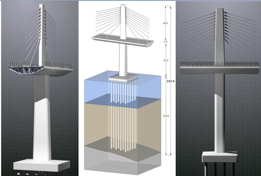
Figure 11. The concept of piers - pylons S5 – S10
