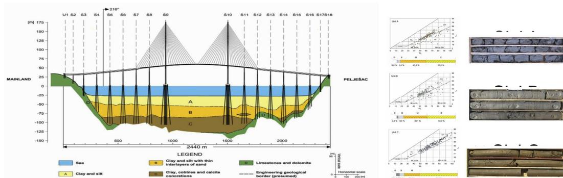
Figure 8. General view of foundation soil characteristics
