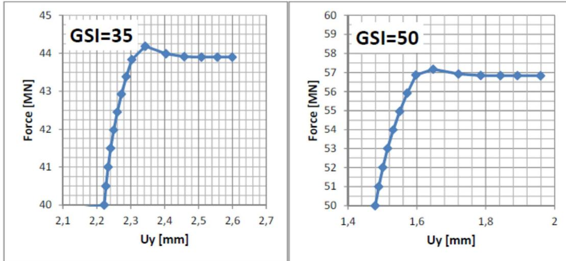
Figure 20, 21. The GSI illustration shows the displacement of the pile toe at failure (GSI=35) and force - displacement curve for the last loading step 40 MN – 50 MN (GSI=35) and 50 MN – 60 MN for GSI=50.
