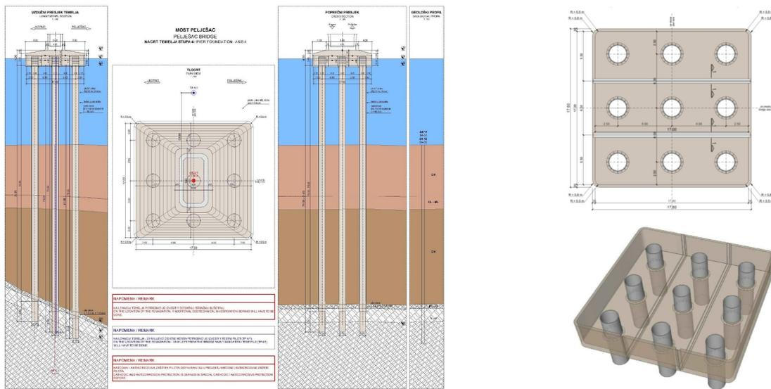
Figure 12. Foundations of piers S3, S4, S11, S12
