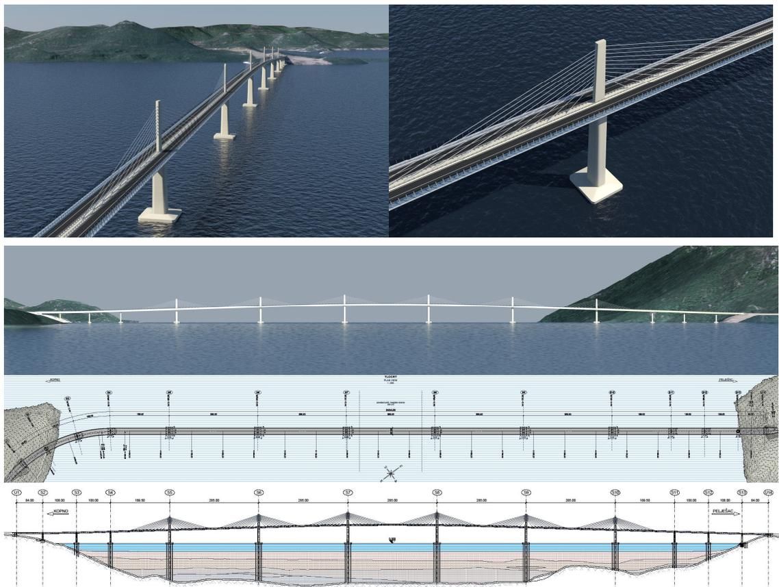
Figure 10. View of the bridge, plan view and longitudinal section
