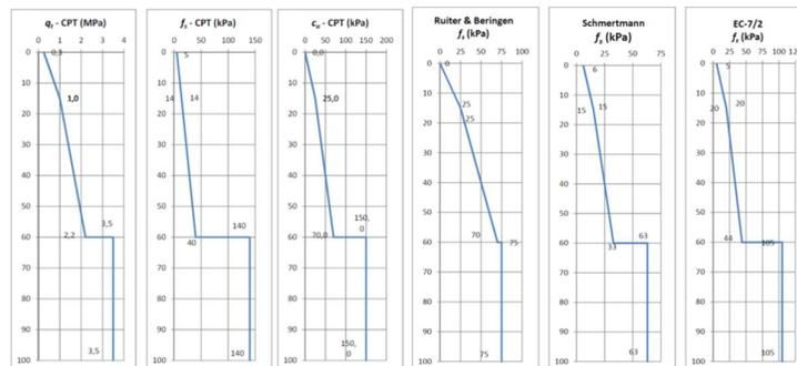
Figures 18, 19. The value of cone tip penetration resistance (CPT)  $q_t$ , shaft friction  $f_s$  and undrained shear strength  $c_u$  vs. depth, Limit value of pile shaft friction  $f_s$  according to Ruiters & Beringen (1997), Schmertmann (1978) and EC 7/2
