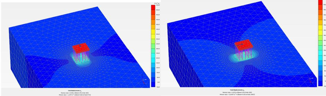
Figure 16. Structural deformations (vertical load + horizontal load 50 MN in the direction of bridge axis and transversely to bridge axis (undrained conditions))
