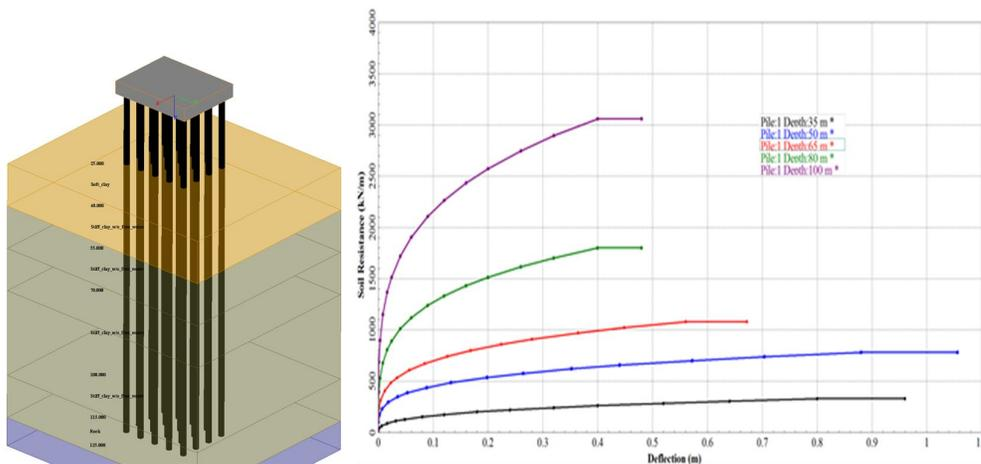
Figure 17. View of "p-y" curves / nonlinear behavior of foundation soil - clay at different depths
