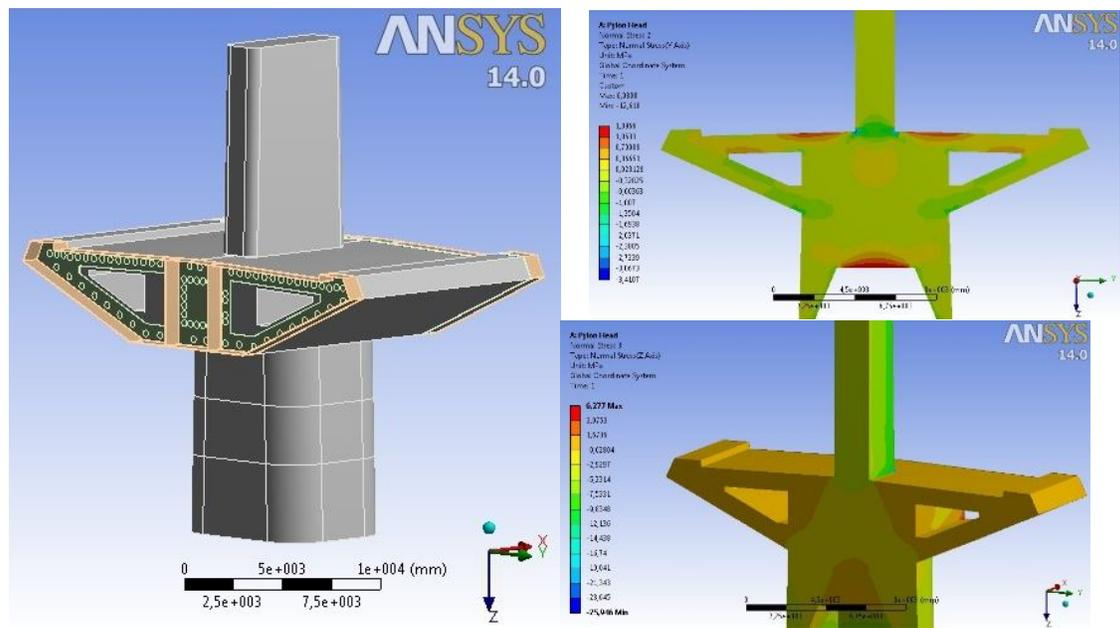
Figure 35. A view of the detailed analysis of the connection of pier, pylon and steel structure with solid elements
