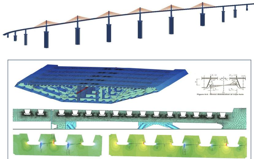
Figure 33. Model of the entire bridge and illustration of fatigue control in superstructure sheet metals
