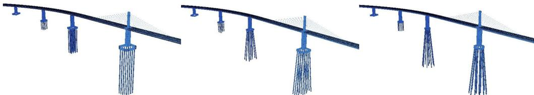
Figure 15. In the stage of searching for optimum foundation engineering method, numerous variants were analyzed with different numbers of piles and with inclined piles.
