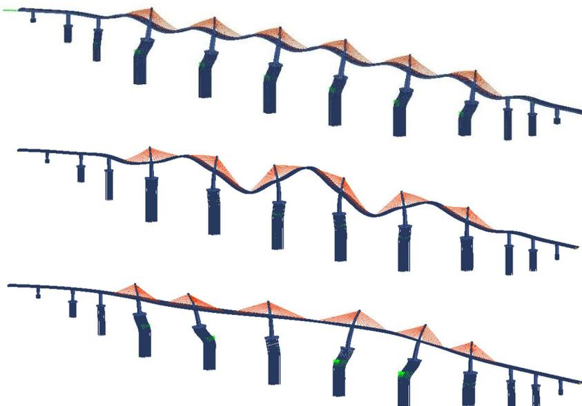
Figure 25. First three oscillation forms of the bridge structure
