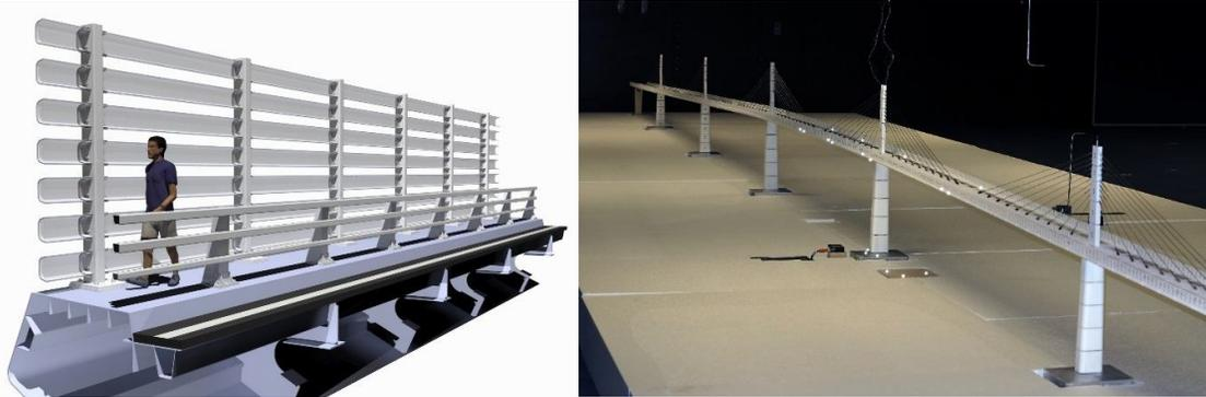
Figures 31, 32. Wind protection fence and bridge model testing (Full Bridge Model Test, 1:150) in the wind tunnel of Force Technology / Copenhagen - Denmark
