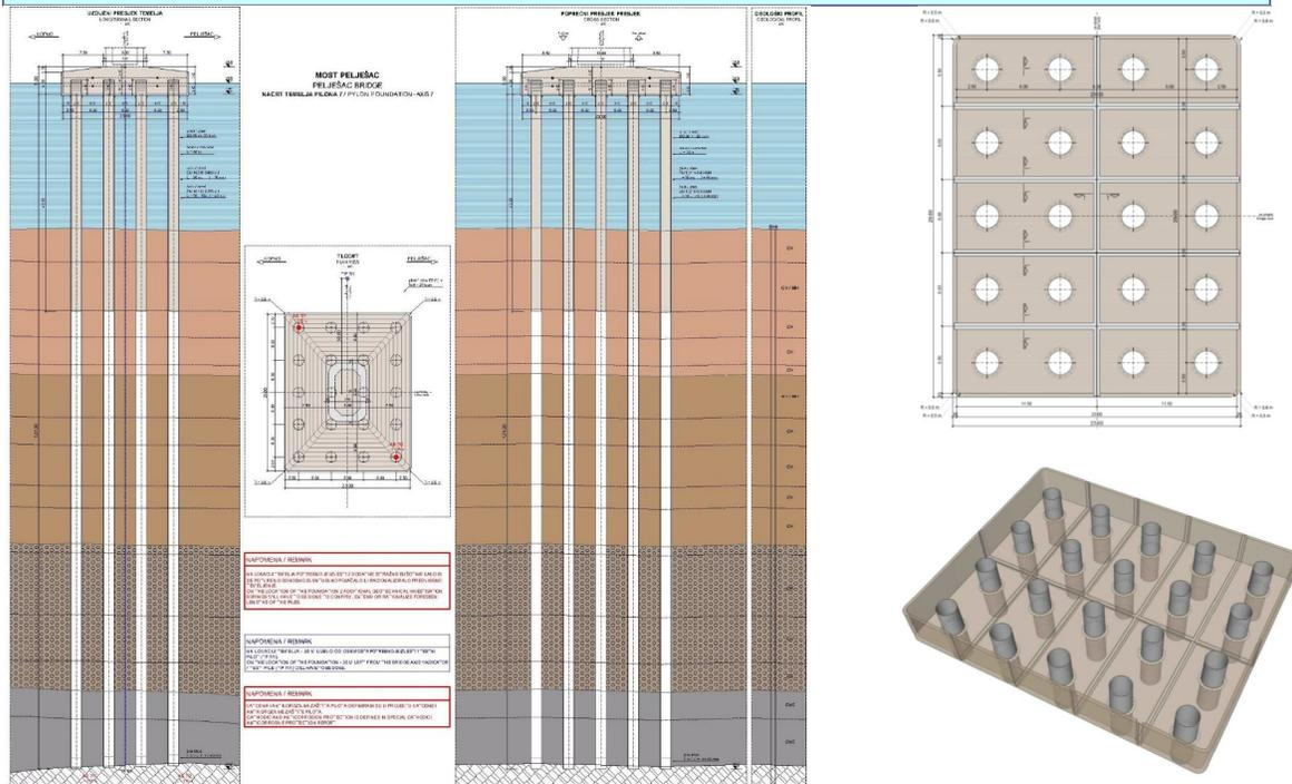
Figure 13. Foundations of piers S7 and S8
