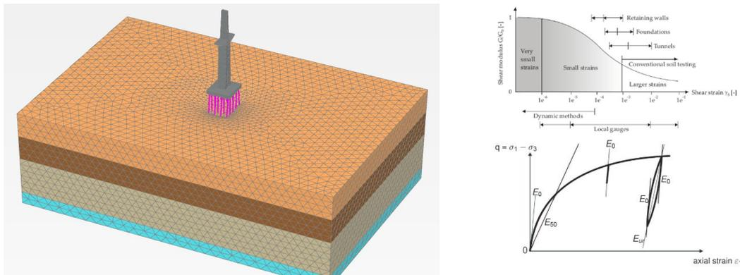
Figure 14. 3D model of the continuum of soil and foundation structure with volume FEM elements
