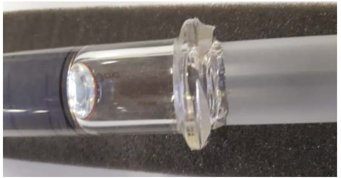
Figure 3. Special sealing between the piston and glass body made to avoid hydrogen escaping from the syringe
