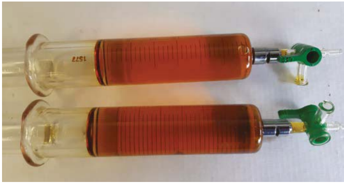
Figure 2. Sampling in duplicate helps reveal incorrect sampling
