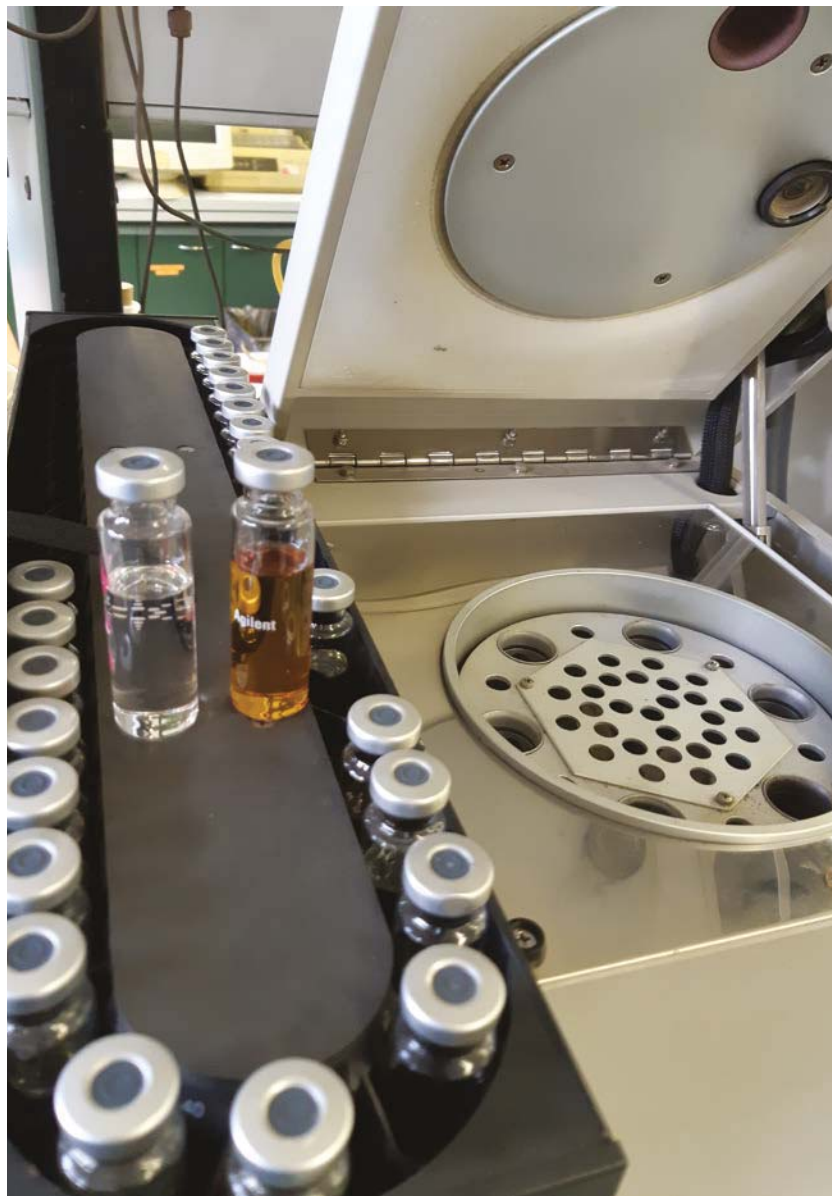
Figure 4. Head Space carousel and the oven for shaking and heating the vials containing the oil sample
