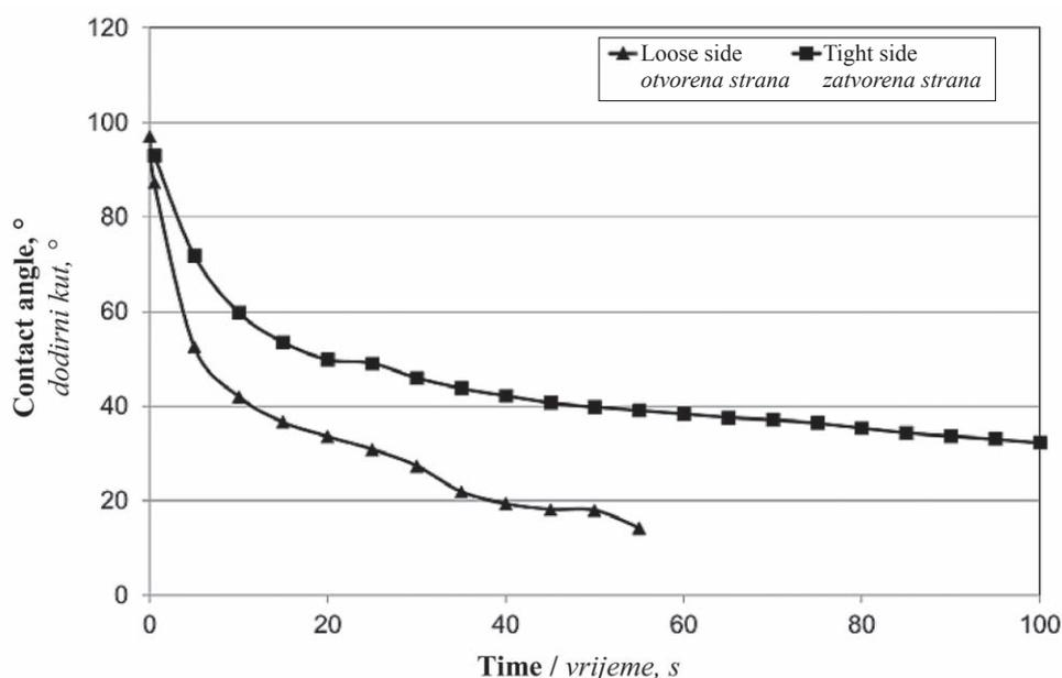
**Figure 1** Changes in dynamic contact angle of distilled water as a function of time on non-densified veneer surfaces
