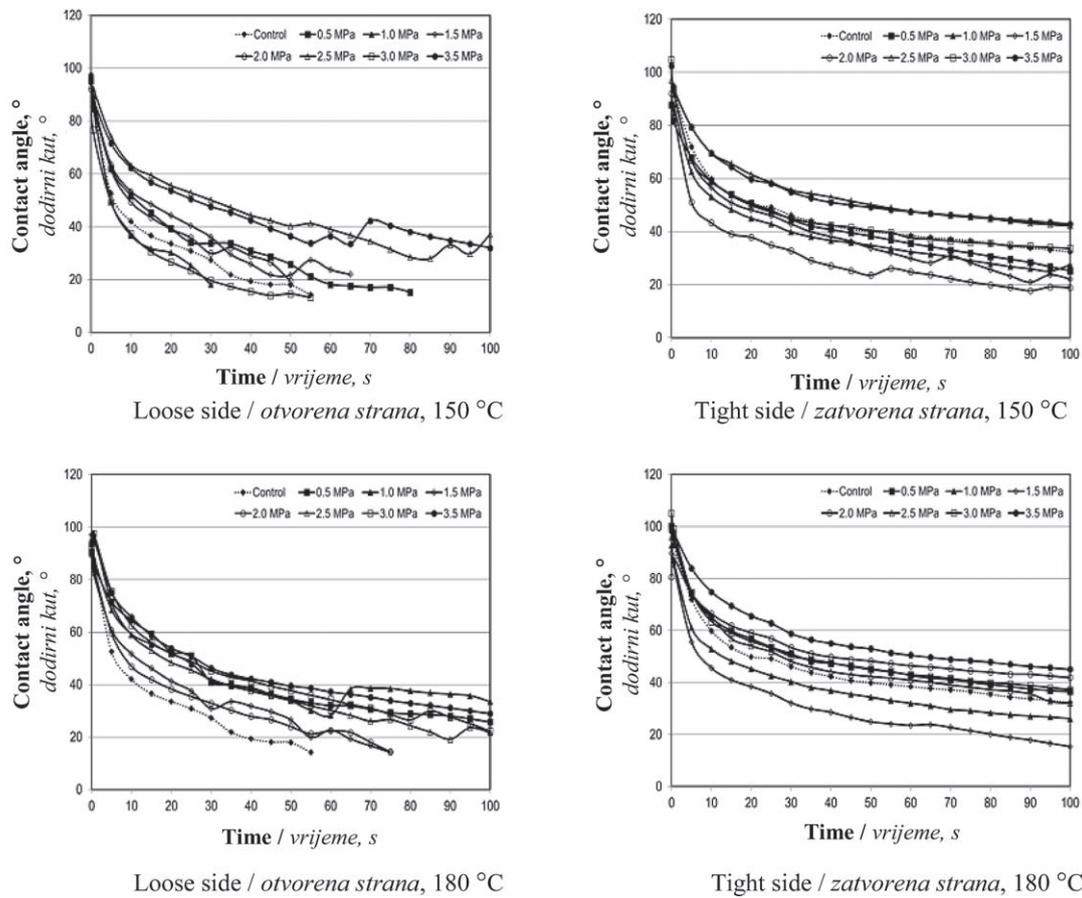
**Figure 2** Changes in dynamic contact angle of distilled water as a function of time on densified surfaces of birch veneer at various compression temperature and pressure values
