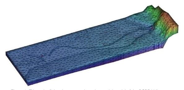
Figure 6. Triangular finite element mesh on the spatial model of the PSPP Vrilo area.
