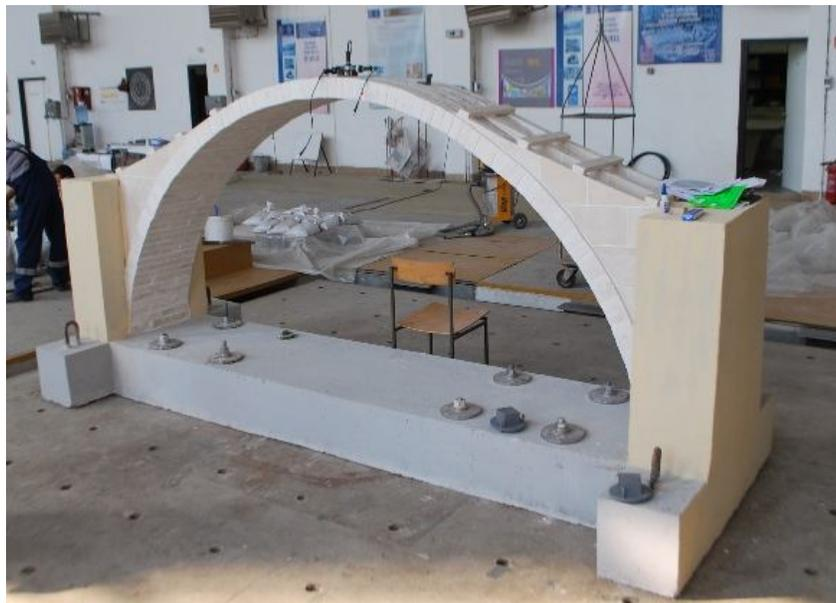
Figure 11. The model of Old Bridge at scale 1:9
