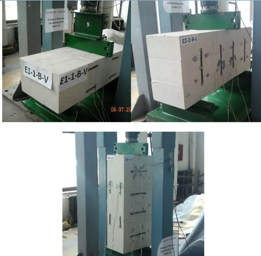
Figure 5. Constructed masonry segments placed in position for testing
