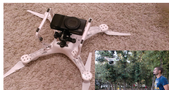
Figure 1: Dji Phantom2 mounted with a RicohGR compact digital camera, author: M. Vuković; Lower right corner - UAV mid-flight, author: M. Doneus
