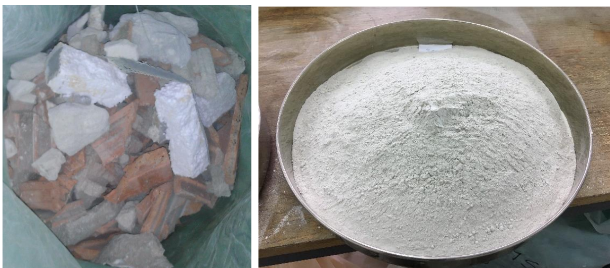
Figure 2 Material for preparation of filler F1 (left) [21] and F32 — fraction 0.063–0.125 mm (right) [22]
