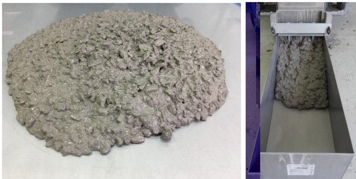
Figure 3 Mixture M10 (slump-flow) [22] and M1 (L-box) [21]
