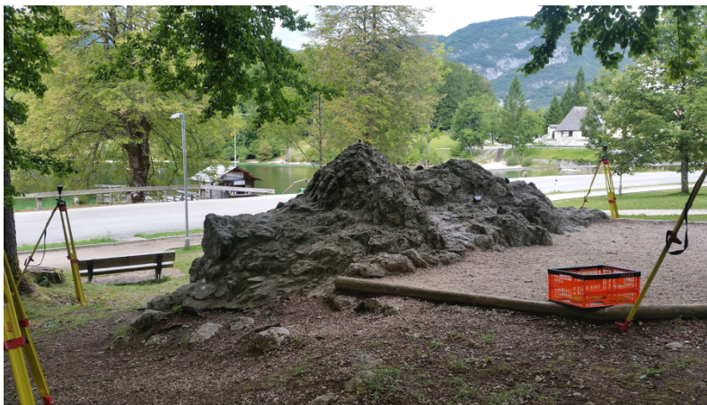
Fig. 3 Stone model of Mount Triglav at the time of survey (by Anita Anželak); marker for reference points; geodetic network around the model.
