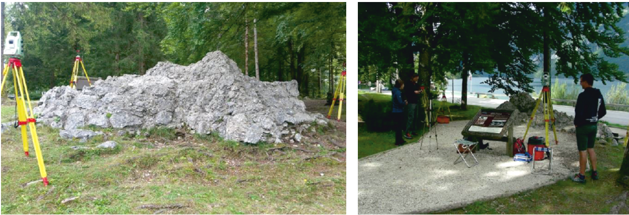
Fig. 4 Terrestrial laser scanning of the stone model with the Leica Nova MS50 instrument (by Anita Anželak - left and Dušan Petrovič - right).
