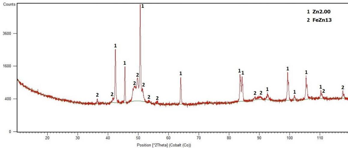
**Figure 1.** The XRD pattern of the phase analysis
