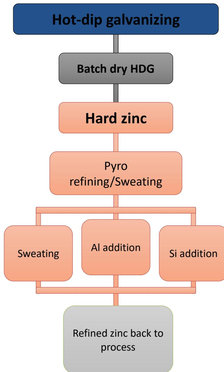
**Figure 5.** The proposal of the experimental part of zinc refining
