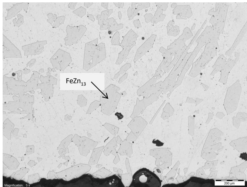
**Figure 2.** Metallographic observation of hard zinc (200x magnification)
