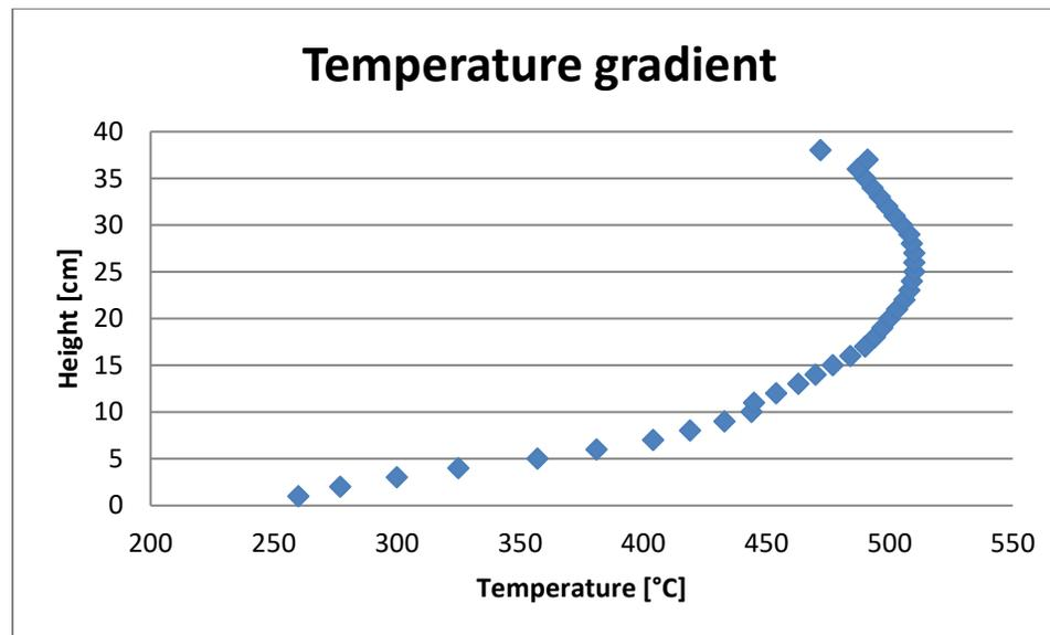
**Figure 4.** Measurement of the temperature gradient in the heat aggregate
