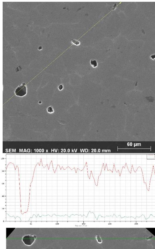
Figure 7. The EDS line scan of sample 2.
