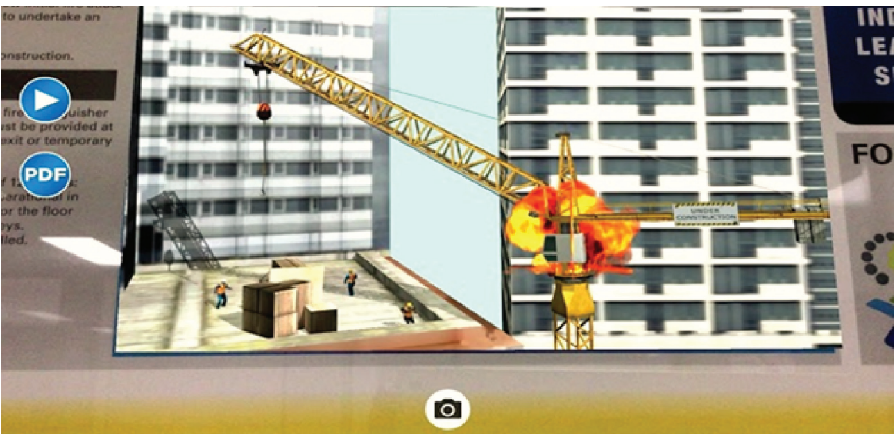
Fig. 6: AR-based construction crane safety application (Pro-Vis AR mobile app).
