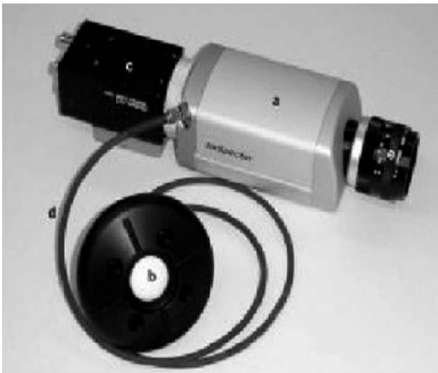
Fig. 1. ImSpector V9 with an insolation collecting unit (FODIS), [5]
