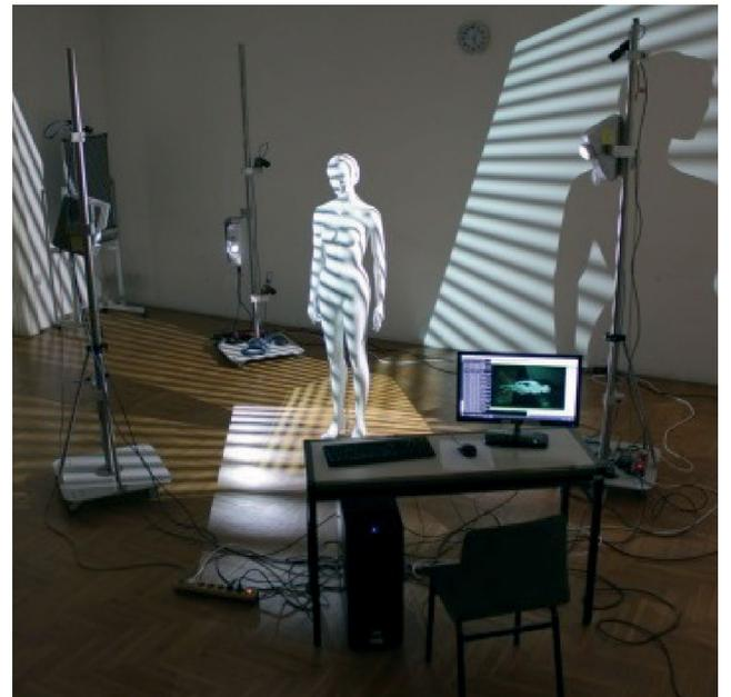
Fig. 1. Our 3D scanning system. Note the inter-projector interference pattern on the mannequin and on the floor
