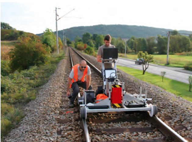
Fig. 2. Conduction of multi-channel GPR investigations within DestinationRAIL project
