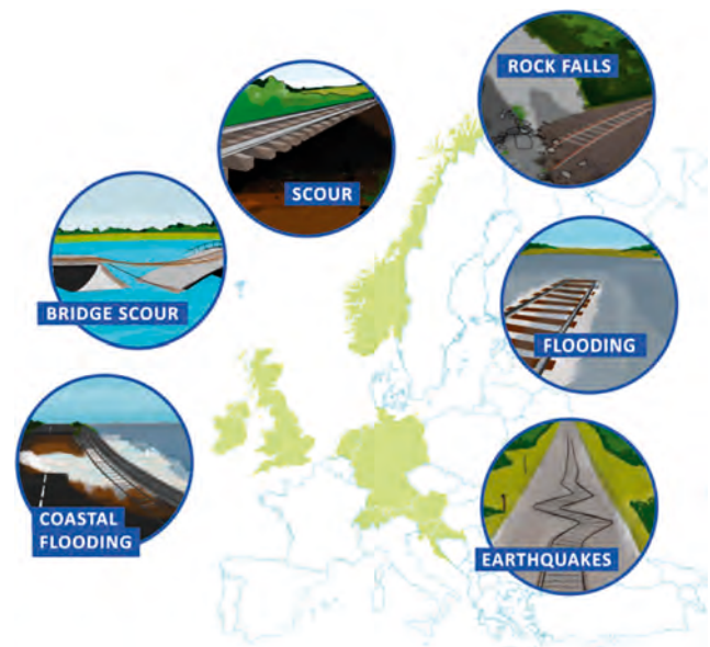
Fig. 1. Different types of failure on railway infrastructure [10]
