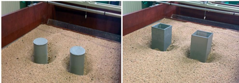
**Fig. 11** – Local erosion around two circular and square piers after achieving the equilibrium condition in experiments 6 and 15 on the physical model (see Table 1)
