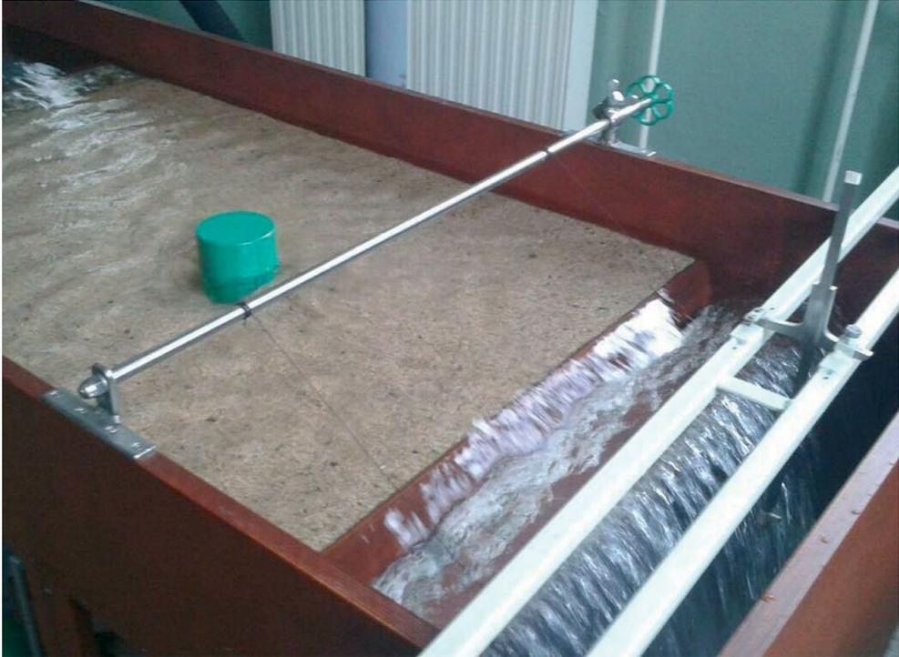
**Fig. 1** – Physical model for local erosion analysis around the pier
