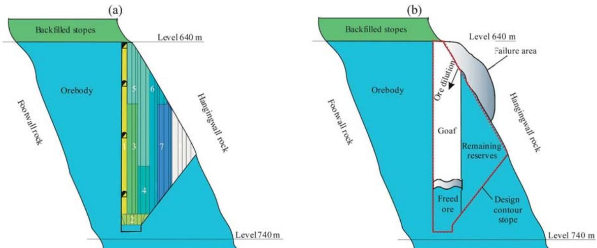
**Figure 2:** Schematic diagram of ore dilution with hangingwall rocks in the chamber: (a) the order of ore extraction in the chamber; (b) ore dilution from the chamber on junction with hangingwall; 1 – 8 numerical order
