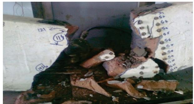
Figure 18 Ultimate failure of partially prestressed reinforced baked clay beam B2
