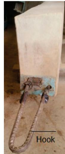
Figure 7 A hook is welded with reinforcing bars of the beam
