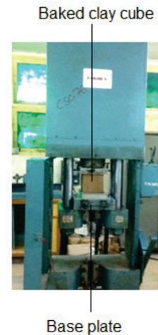
Figure 10 Baked clay cubes are being compressed in the Universal Testing Machine to determine compressive strength
