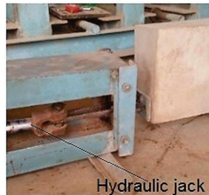
Figure 8 Steel reinforcing bars are being partially prestressed using hydraulic jack
