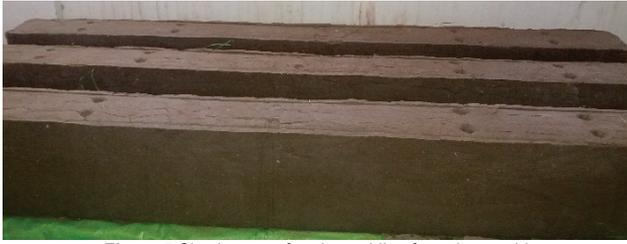
Figure 5 Clay beams after demoulding from the mould
