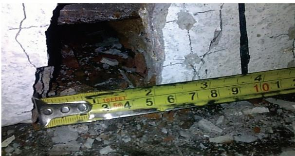
Figure 15 Widening of initial crack at midspan of partially prestressed reinforced baked clay beam B1
