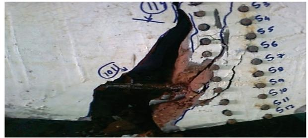
Figure 16 Widening of initial crack near midspan of partially prestressed reinforced baked clay beam B2
