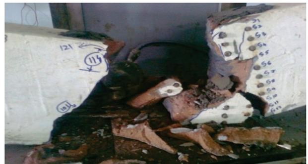
Figure 18 Ultimate failure of partially prestressed reinforced baked clay beam B2
