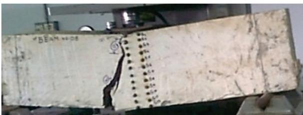
Figure 14 Opening of initial single crack near midspan of partially prestressed reinforced baked clay beam B2
