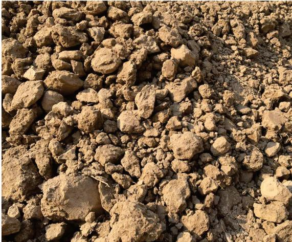
Figure 1 Lumps present in excavated clay
