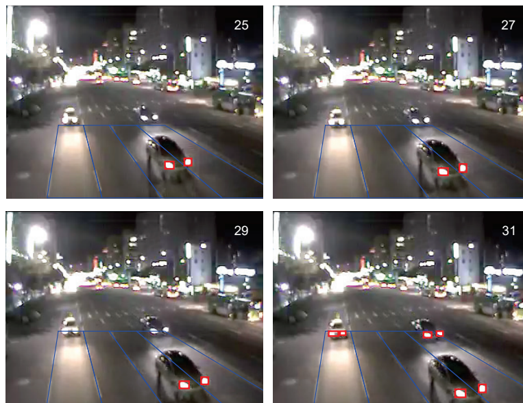
Figure 7 Examples of detected vehicles in terms of individual headlight
