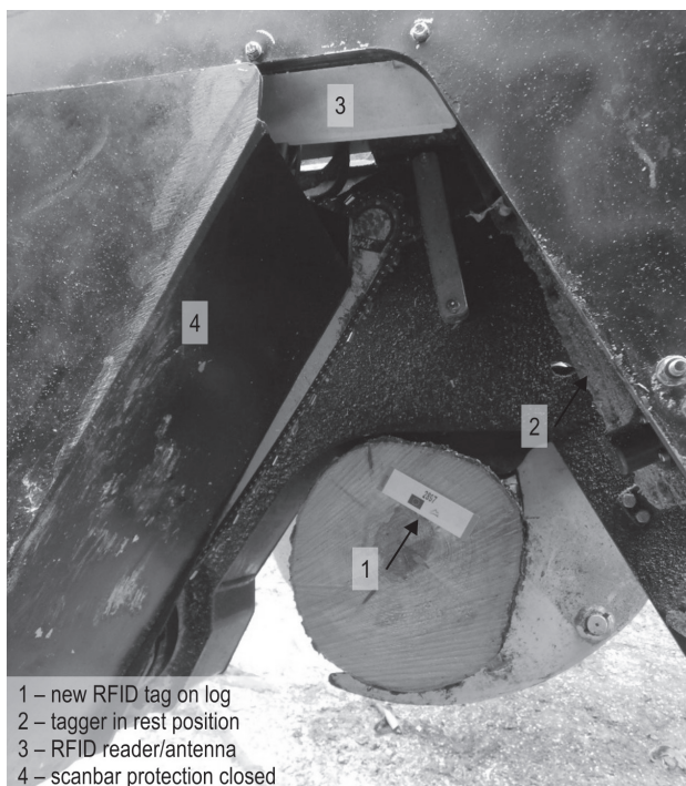
Fig. 10 Identification of the new RFID tag applied by the tagger
