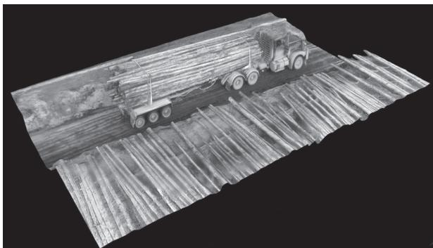
Fig. 6 Tile model generated with Agisoft PhotoScan
