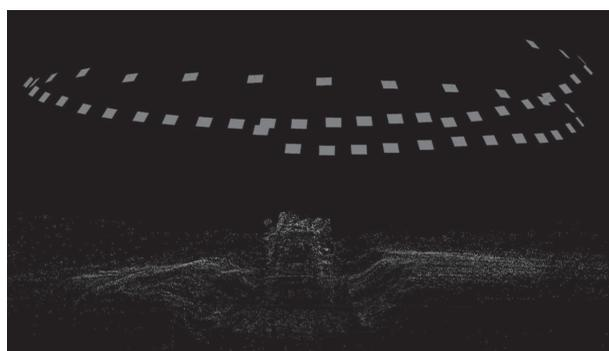
**Fig. 3** Sparse point cloud generated with Agisoft PhotoScan
