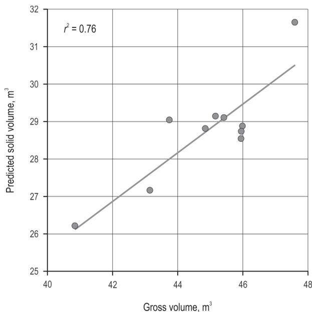
**Fig. 8** Regression model between gross and predicted solid volume of logs on trucks
