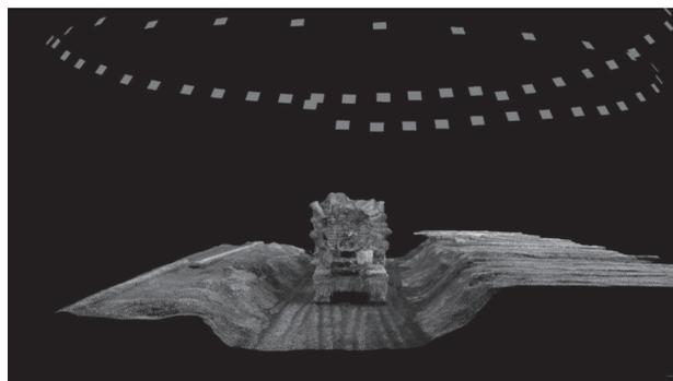
Fig. 4 Dense point cloud generated with Agisoft PhotoScan
