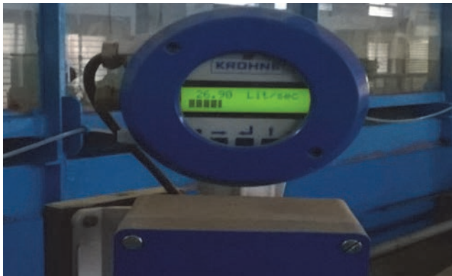
Figure 6. Photograph of electromagnetic flow meter used in experiment
