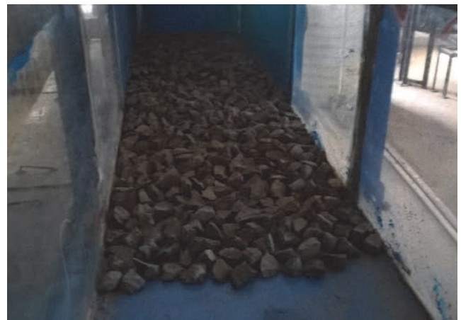
Figure 3. Photograph of crushed stones glued onto flume bed to form rough bed for experiment
