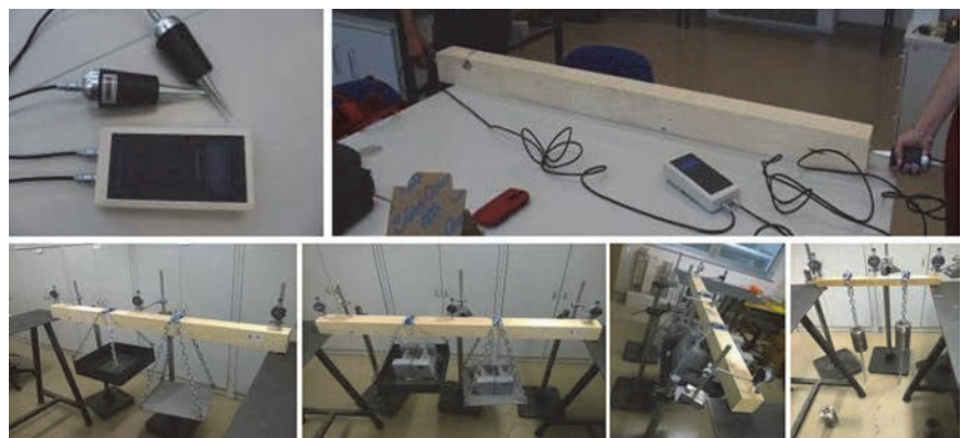
Figure 3. ND tests – a) ultrasonic stress-wave (longitudinal) test (phase 2) i b) static bending test (phase 3)
