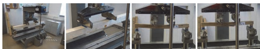
Figure 4. Destructive bending tests (phase 4) and corresponding failure types
