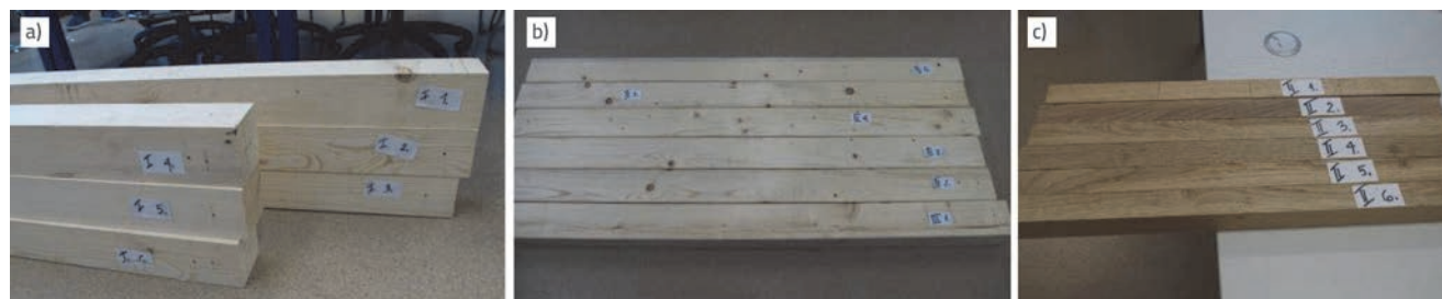
Figure 1. Specimens of structural softwood and hardwood for testing phases from 1 to 4: a) and b) spruce beams (grouped into samples I. and III.); c) oak billets (grouped into II. sample)
