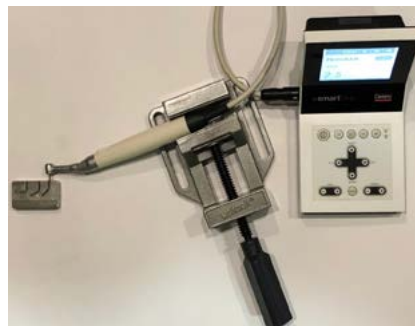
Figure 1. Hyflex EDM 25/~ file in an artificial 60° canal.
