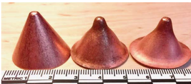
Figure 13: Intact (left) and deformed liners due to partial detonation (middle, right)
