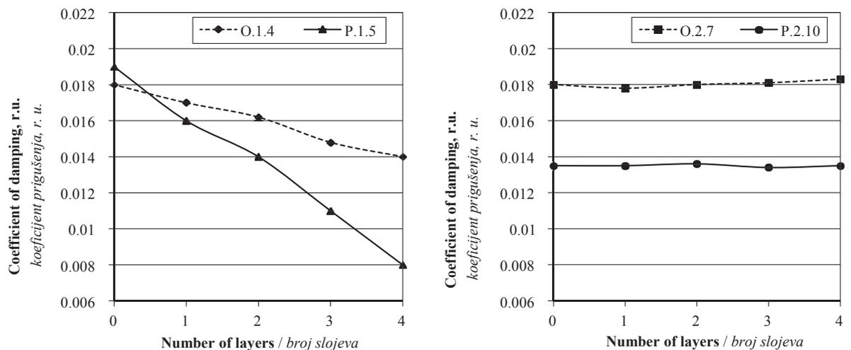
a) b) **Figure 3** Variations of damping coefficient of specimens by increasing the number of layers of the finishing material: a) varnish finish; b) oil finish
