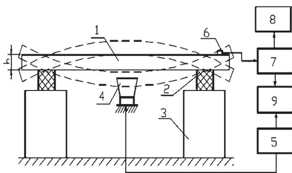
**Figure 1** Scheme of test stand: 1 - specimen; 2 - vibration damping material (foam rubber); 3 - massive supports; 4 - loudspeaker; 5 - vibration generator; 6 - sensor; 7 - measuring instrument; 8 - oscilloscope; 9 - phase meter
