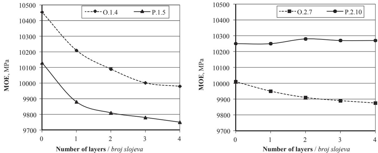
a) b) **Figure 2** Variations of specimens MOE by increasing the number of layers of the finishing material: a) varnish finish; b) oil finish; these are unique identification numbers of specimens –O.1.4, P.1.5, O.2.7, P.2.10.
