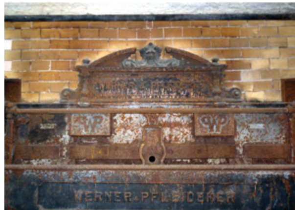
Sl. 14. Detalj sačuvane krušne peći proizvođača Werner & Pfliederer (fototeka HRZ-a, snimila I. Pauk Sili) Details of the preserved brick oven made by Werner & Pfliederer (Croatian Conservation Institute Photo Archives, I. Pauk Sili)
