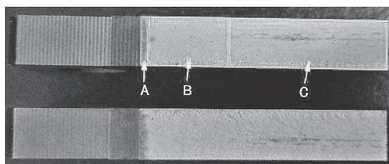
**Figure 5** Fatigue fracture
