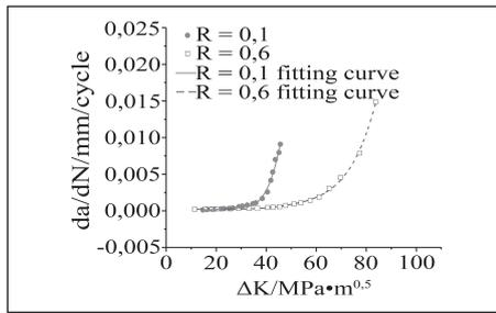
Figure 1 da/dN-ΔK curve
