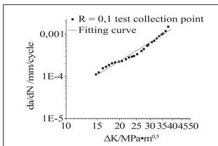
Figure 2 da/dN-ΔK curve for R = 0,1
