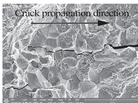
**Figure 6** Extended path of small cracks in the fracture
