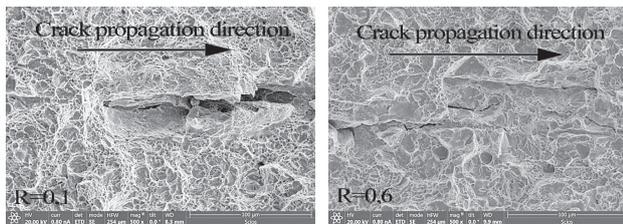
**Figure 7** Dimple state diagram for stress ratios of 0,1 and 0,6
