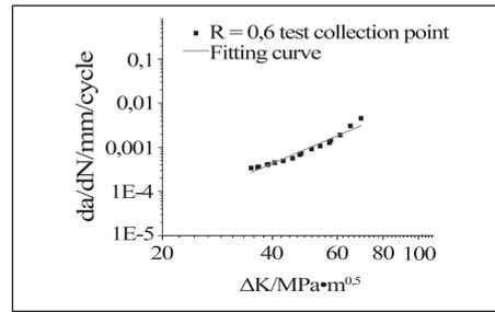
Figure 3 da/dN-ΔK curve at R = 0,6
