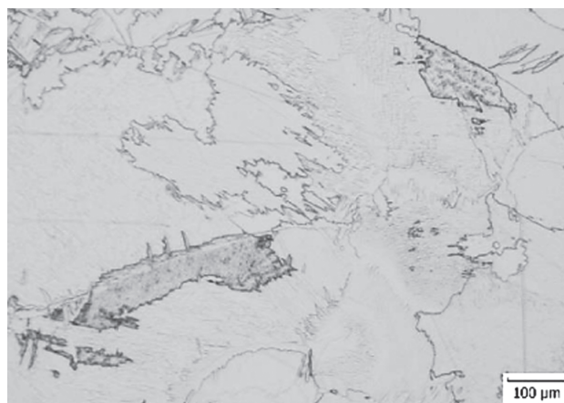
Figure 6 Weld metal microstructure
