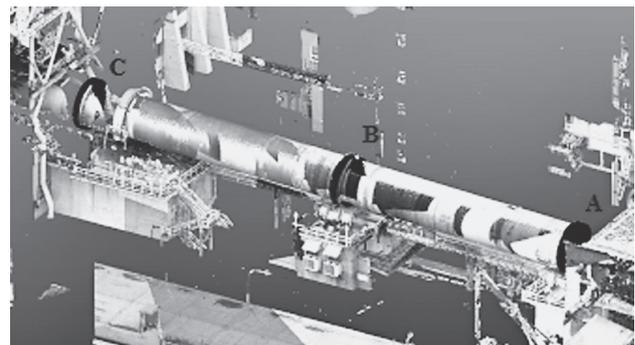
**Figure 2** Carrier tires of the rotary kiln
