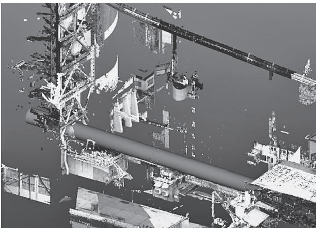
Figure 3 Cylinder with the nominal value of the radius
