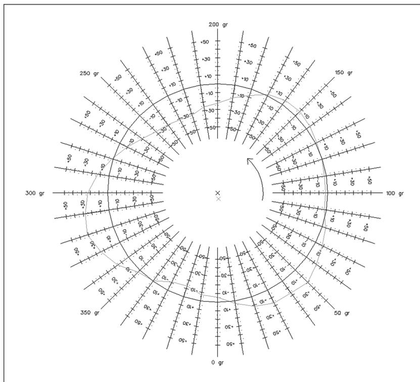
Figure 4 Center graphs - differences between radiuses of the nominal cylinder and real surface of the RK shell
