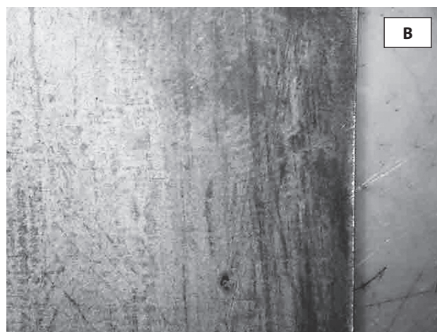
Figure 4 Images of nickel coatings from stereo microscope (A – simple 1, B- simple 20).
