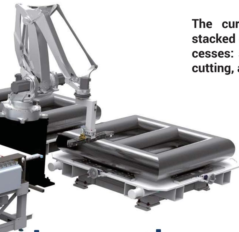
The current production of transformer stacked cores involves three different processes: slitting of core steel sheets, core cutting, and core stacking
