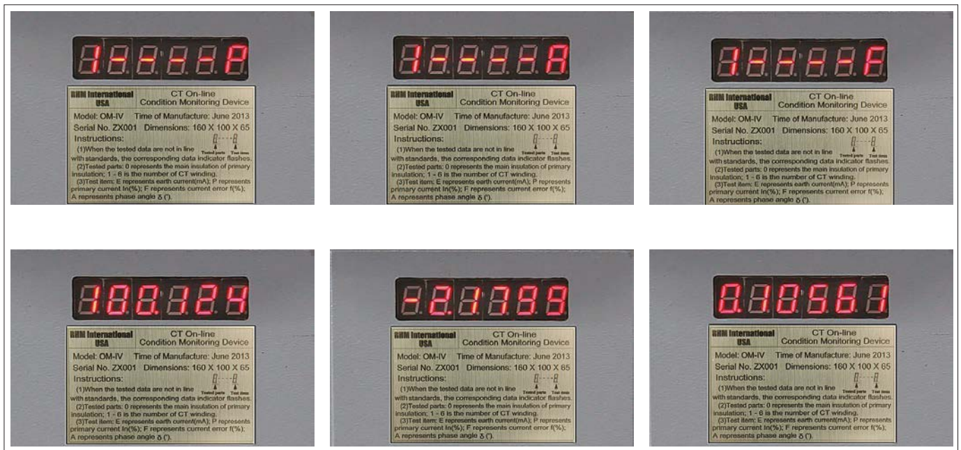
(a) Winding # 1 Operating at 100.124% of the rated current
