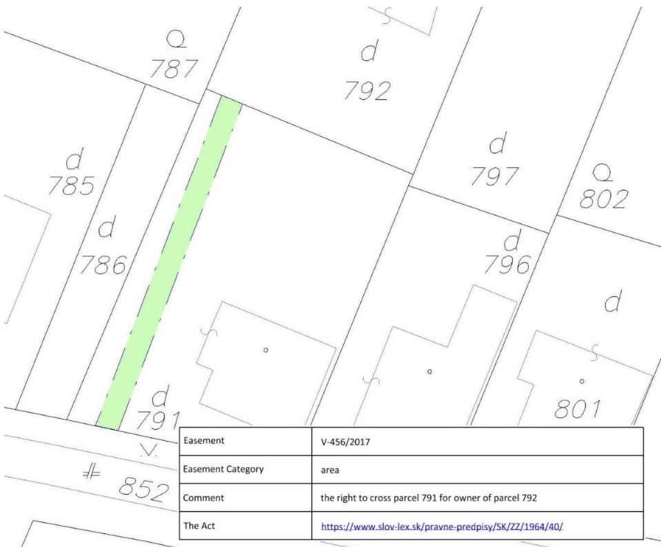
Fig. 3. Displaying of the right to cross a real estate easement on the web portal.
