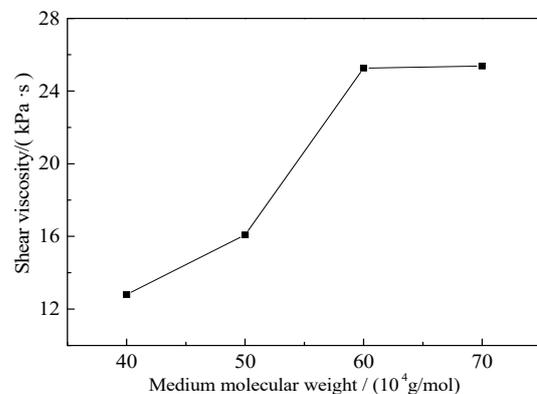
Figure 6. Shear viscosity with different medium molecular weights.
