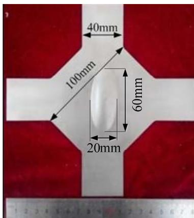
Figure 1. Wrinkling specimen.
