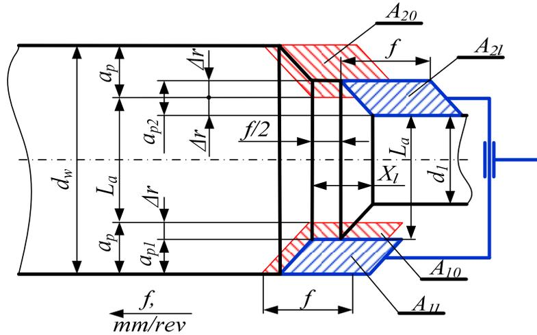
Figure 1. Scheme of turning the MTBB with axially displaced inserts.
