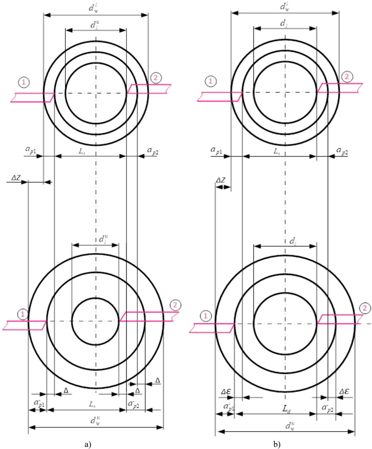
Figure 2. Impact of allowances fluctuations on the diameter of the treated surface: a) with a non-deformable block b) with a deformable block.
