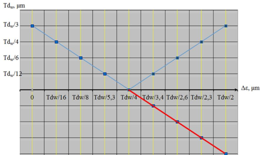
Figure 3. Dependence between the diameter tolerance after turning  $Td_l$  and the stability (elasticity)  $\Delta\varepsilon$  of the MTBB with the axially displaced inserts at a distance of  $X \geq X_1$  expressed by the diameter tolerance of the work piece  $Td_w$ .
