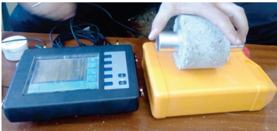
Figure 8 Testing of E modulus by the ultrasound method
