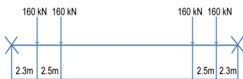
Figure 3 Sketch of train loads' arrangement
