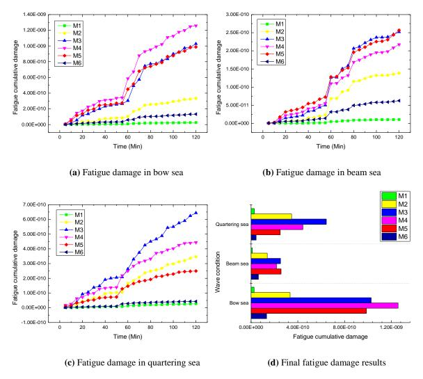
Fig. 19 Transverse fatigue strength assessment
