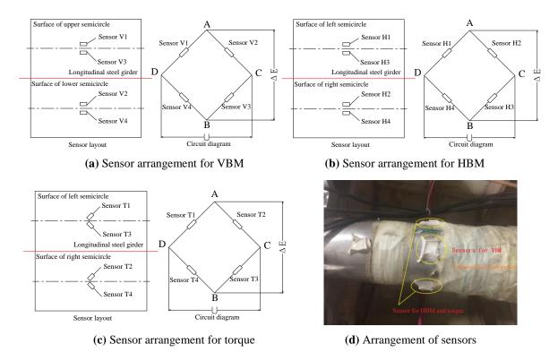
Fig. 10 Arrangement and installation of strain gauges
