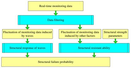
Fig. 5 Process of longitudinal strength evaluation
