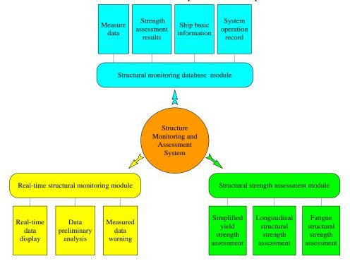
Fig. 1 Scheme of monitoring system
