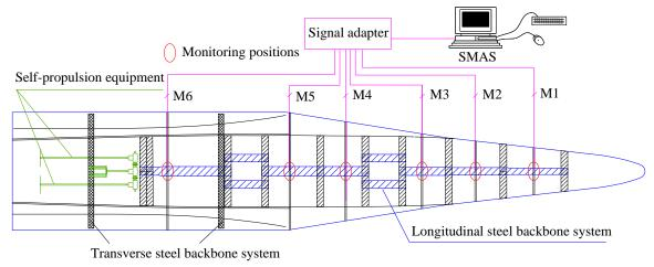
Fig. 9 Design of trimaran model
