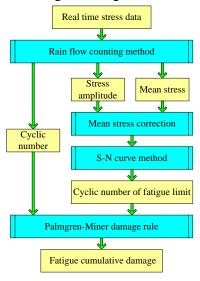
Fig. 6 Process of fatigue strength assessment
