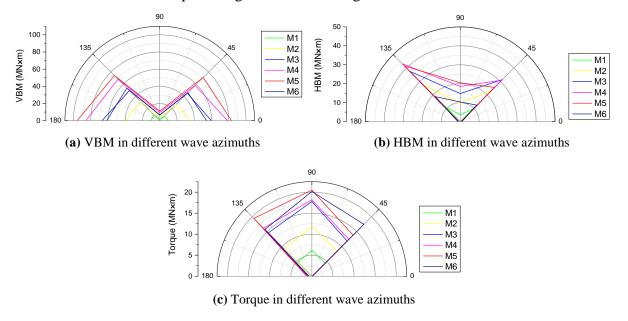
Fig. 14 Structural responses with different wave azimuths
