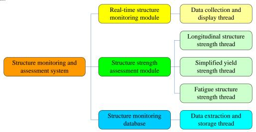
Fig. 2 Multi-threading scheme of monitoring system
